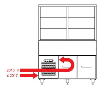
CE mark is located on the right side of the refrigeration unit: EEVA-800, EEVA-1200
